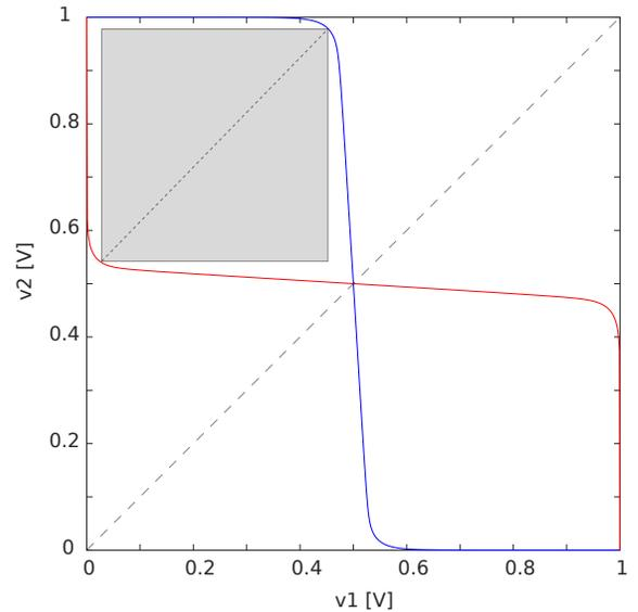
Fig. 2. Butterfly curve, derived from the intercepting of the inverters’ VTC, and the largest possible square enclosed by one of its lobes.
