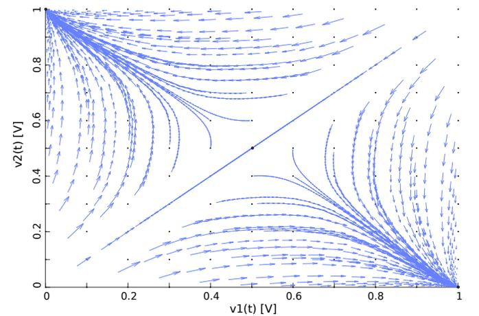
Fig. 8. Trajectories on the space state for an  $11 \times 11$  grid of initial conditions, over  $5ns$  transient simulations.
