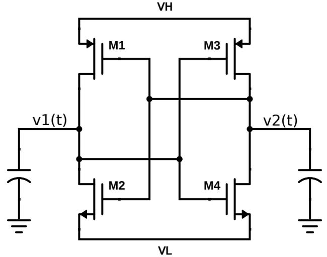
Fig. 5. Non-accessed 6T Static Random Access Memory bit cell.
