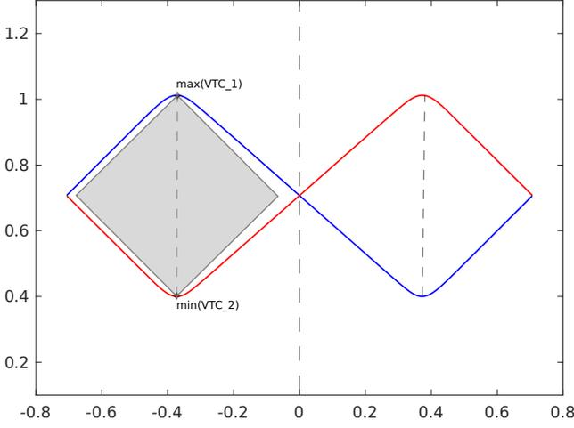
Fig. 3. Rotation of the butterfly curve in vertical alignment to the bisector axis.
