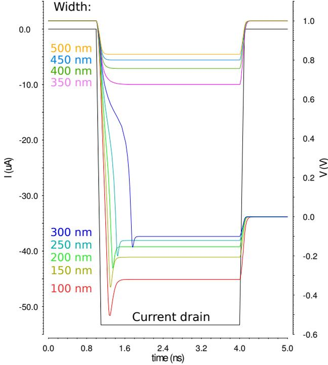
Fig. 6. Dynamics of the SRAM bit cell for a draining current applied to the input of the inverter loop.
