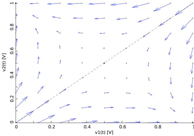
Fig. 9. Bit cell's space state dynamics in light of a vector field, given a 9x9 grid of initial conditions.
