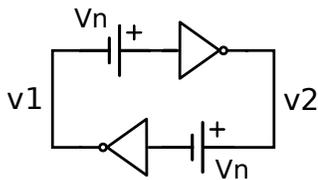
Fig. 1. Closed-loop configuration of two back-to-back connected inverters.
