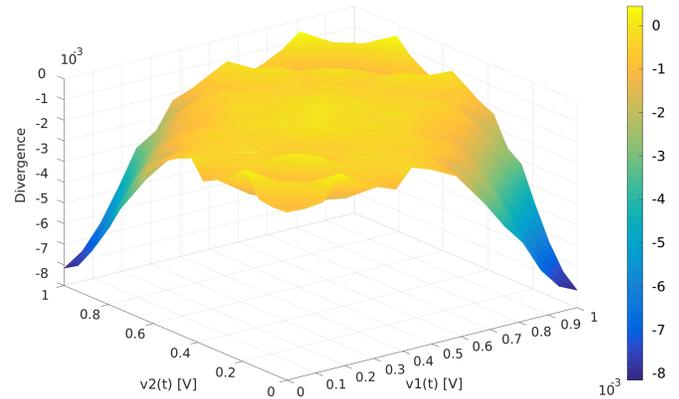
Fig. 10. Divergence of the space state vector field for the non-accessed 6T SRAM bit cell.
