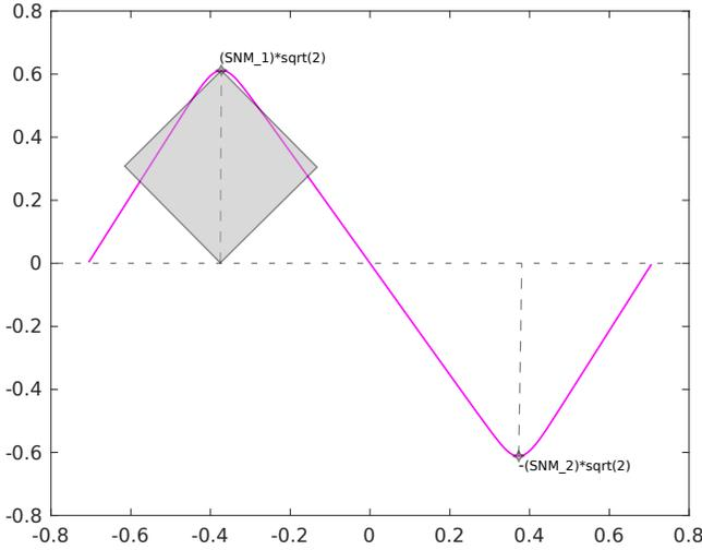
Fig. 4. Subtraction of  $VTC_1$  by  $VTC_2$ , capturing maximum and minimum values of the resulting curve in accordance to the squares' diagonal lengths.
